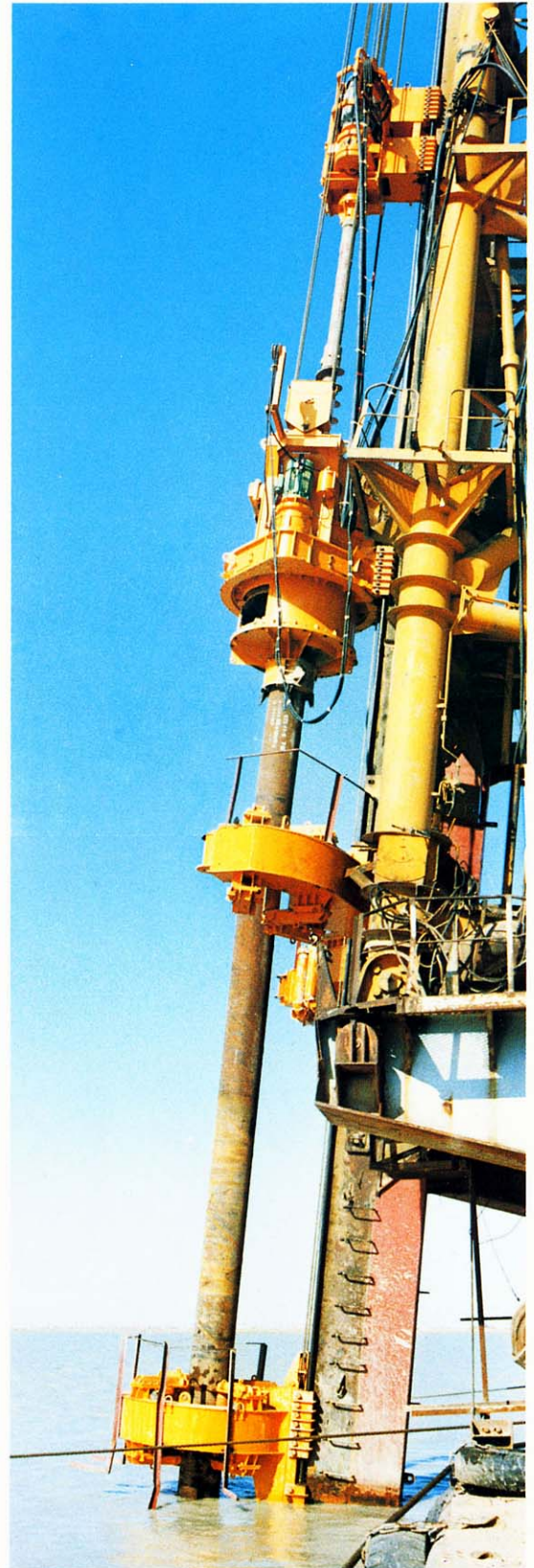
Doughnut Auger Model SDA-180P mounted on the barge Leader length: 34.5M
