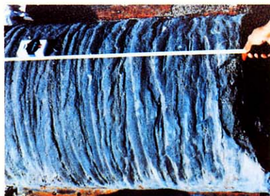
Tested Sample of Consolidation mixed with Cement Milk and Reclaimed Soil
