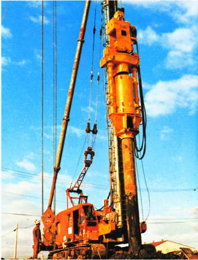
SANWA AUGER MODEL D-60H FOR AUGER-CAISSON PILING METHOD
